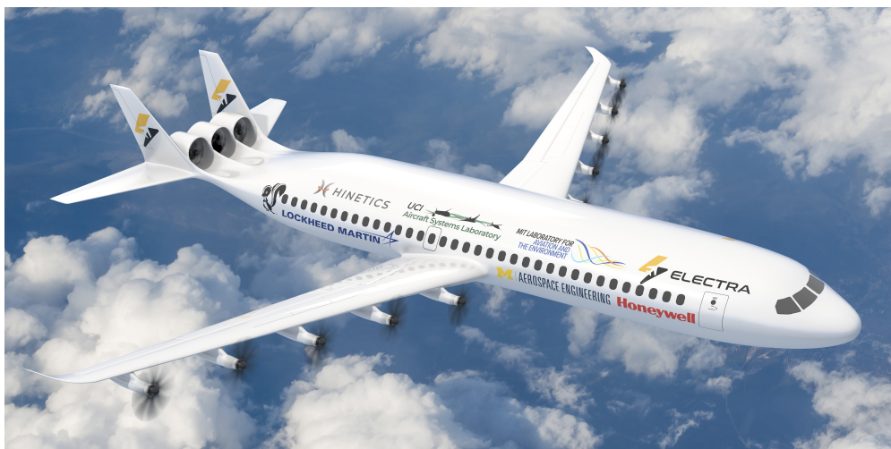
Figure 1: Concept aircraft illustrating the advanced technologies being modeled, including electrified propulsion, distributed propulsion, boundary layer ingestion, and blown lift. It serves as a research baseline and does not represent an optimized future configuration.
