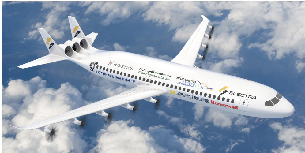
Fig. 1 Concept aircraft illustrating the advanced technologies being modeled, including electrified propulsion, distributed propulsion, boundary layer ingestion, and blown lift. It serves as a research baseline and does not represent an optimized future configuration.
