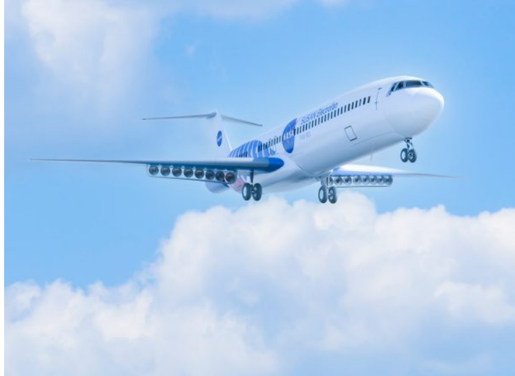
Fig. 1 The Subsonic Single Aft Engine (SUSAN) aircraft concept, published by NASA [5].
